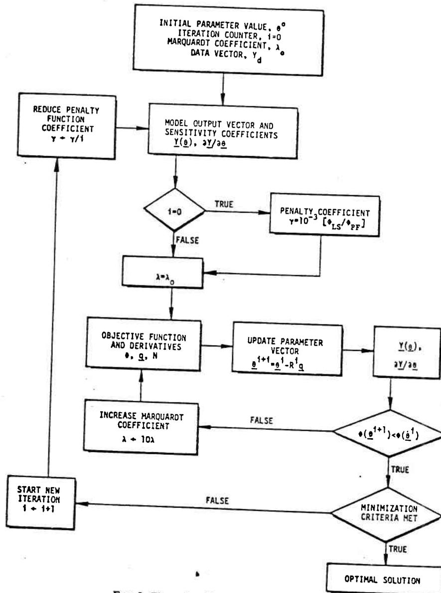
FIG. 3. Flow chart for optimization algorithm.
