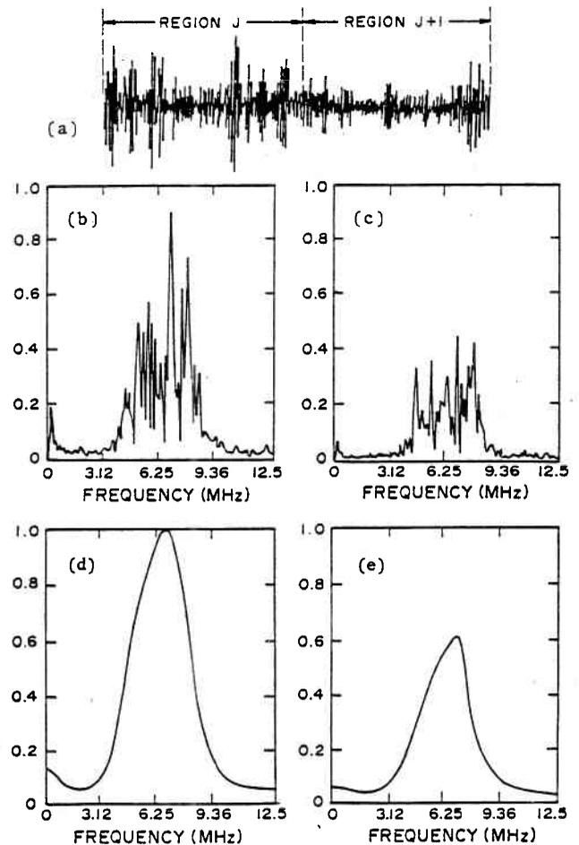
FIG. 3. (a) A typical grain signal; (b) and (c) magnitude spectra of regions  $j$  and  $j + 1$ , respectively; (d) and (e) cepstral smoothing of magnitude spectra of regions  $j$  and  $j + 1$ , respectively.
