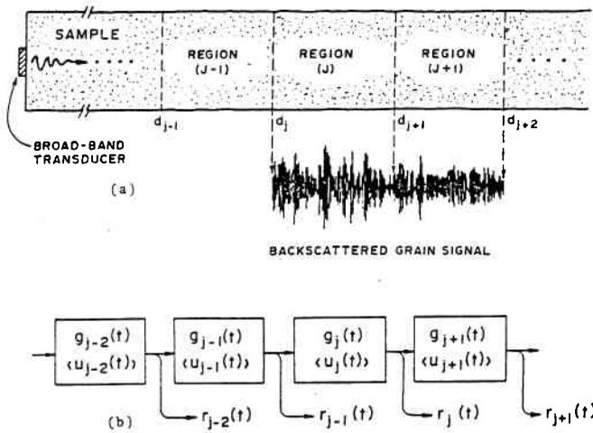
FIG. 1. A sample under ultrasonic testing for grain size estimation using backscattered echoes. (a) A typical backscattered grain signal corresponding to region  $j$  and  $j + 1$ ; (b) segmented model of the backscattered grain signal.
