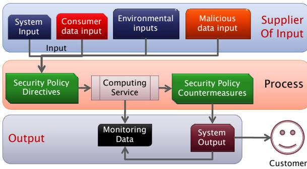
Figure 4. Security SIPOC chart of a computing process.
