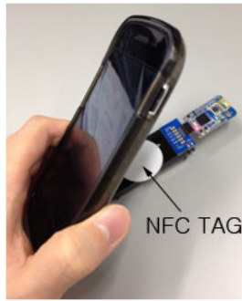
Figure 2. Initiating connection process
