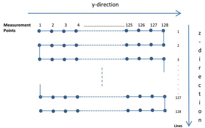
Figure 4. Scanning pattern of the transducer for 3D ultrasonic data acquisition
