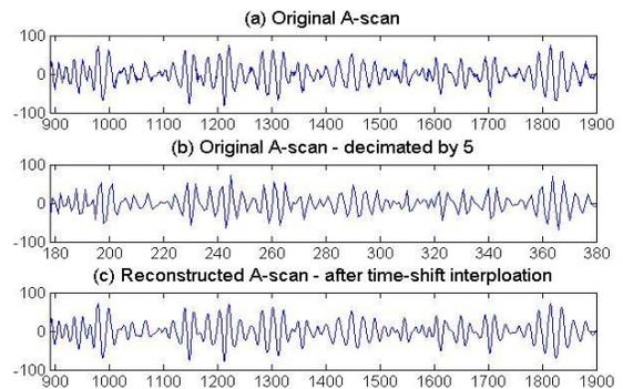
Figure 1. 80% Compression by decimation and reconstruction by time-shift interpolation
