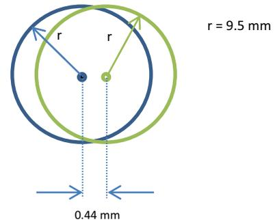
Figure 5. Transducer cross-section at two sample points
