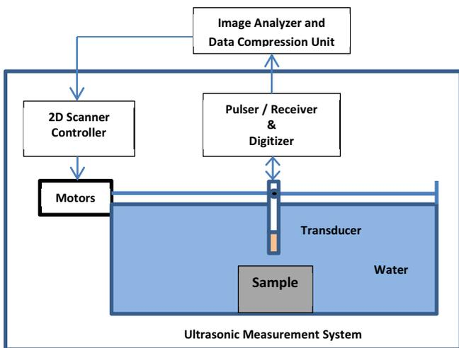
Figure 3. Ultrasound data acquisition setup
