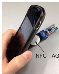
Figure 3. NFC tagging procedure for Android application execution
