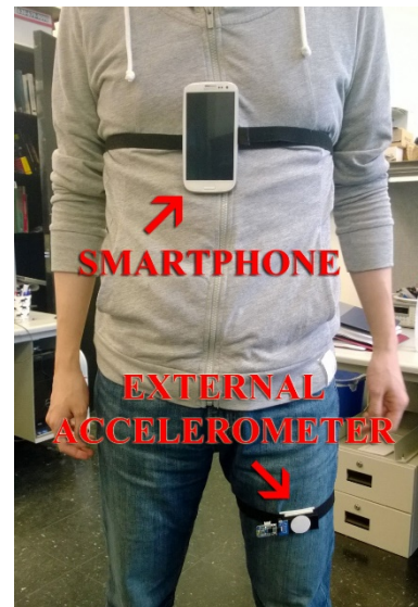
Figure 2. Example of a wearable system configuration with smartphone and external accelerometer
