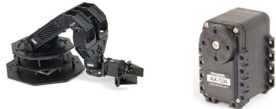
Figure 2. Phantom X Reactor robotic arm (left) and Dynamixels AX-12A (right)
