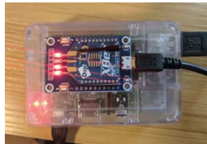
Figure 4. Personal Communication Node using ZigBee-enabled Raspberry Pi
