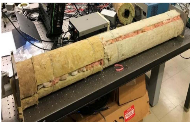
Figure 2. Mineral wool thermal insulation installation
