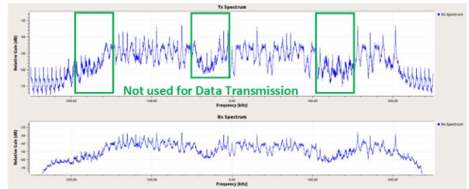
Figure 4. OFDM Transmitted and Received Baseband Signal Frequency Response in real-time Ultrasonic Communication on SDUC
