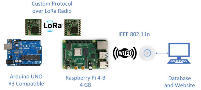
Figure 6. Overview of Prototype System Connectivity
