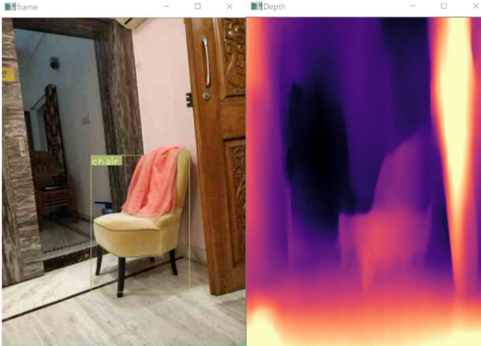
Figure 6. Sample Image and Depth Map Obtained from IP Webcam Feed
