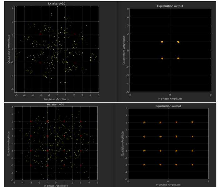
Fig. 5. The Constellation of Rx Signals Before/After Equalization.
