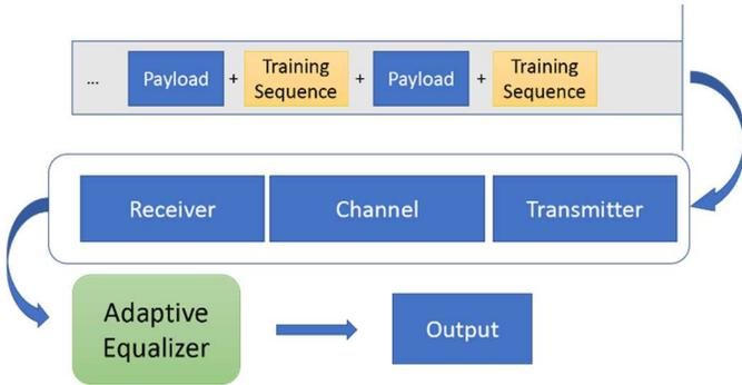
Fig. 3. Data Flow of the Adaptive Equalizer.
