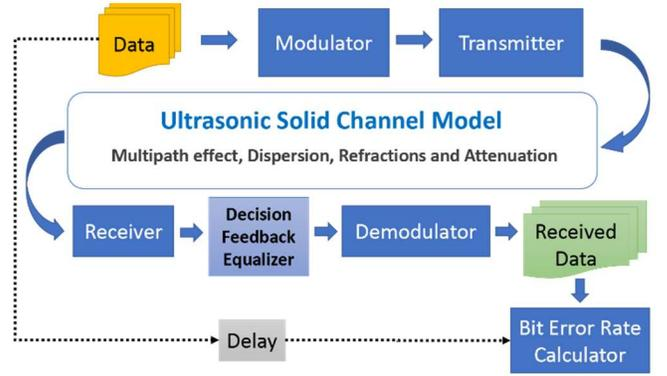
Fig. 4. System Diagram of the Equalization and BER Estimation.
