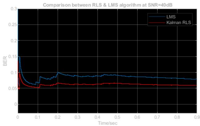
Fig. 6. Bit Error Rate Comparison of LMS and RLS
