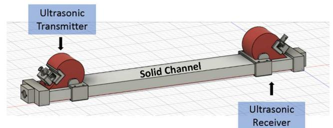
Fig. 1. The Layout of the Solid Channel Communication.
