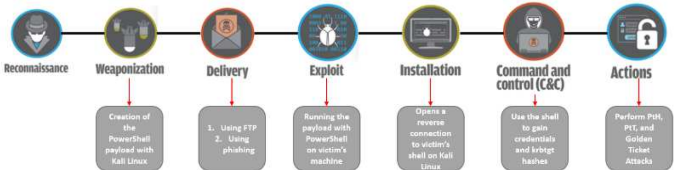
Fig. 1. Cyber Kill Chain for the successful acquisition of Kerberos hashes to compromise the Kerberos authentication mechanisms.
