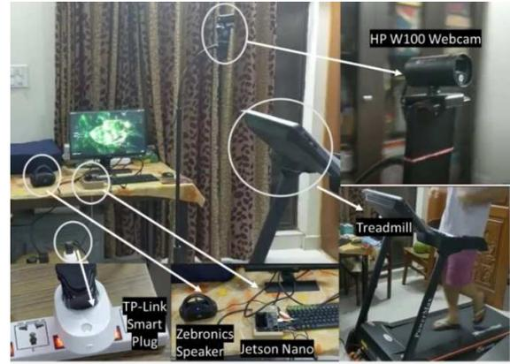
Figure 12. Treadmill Safety System Prototype
