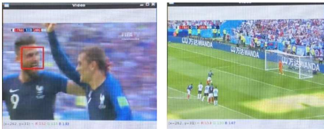
Fig. 2. Dlib Face Detection Results of Zoomed-In View (left) and Aerial View (right)
