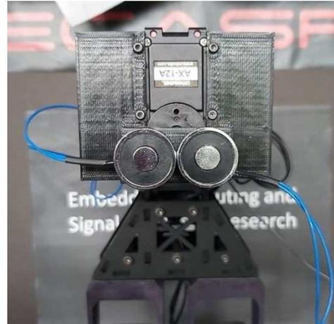
Fig. 4. 3D-Printed Magnet Support with two electromagnets mounted.
