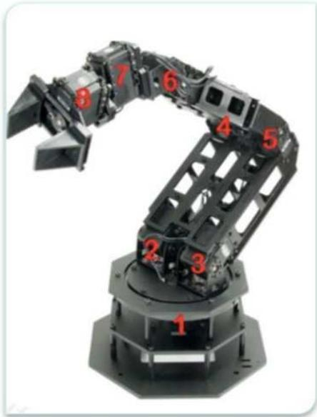
Fig. 3. Motor distribution on the robotic arm
