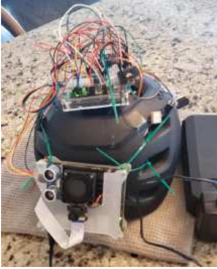
Fig. 5 Picture of Implemented Smart Bike Helmet
