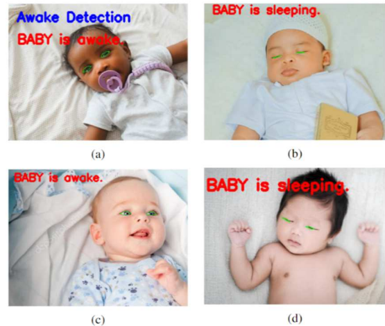
Fig. 8. Result for awake detection. (a) Baby is awake (EAR=0.29), (b) Baby sleeping (EAR=0.11), (c) Baby is awake (EAR=0.35), (d) Baby is sleeping (EAR =0.14).
