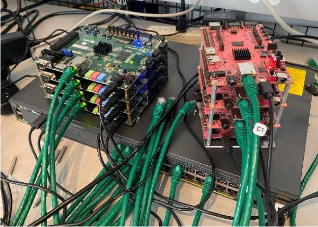
Fig. 1. FPGA Stack with Four ZedBoards and Four PYNQ-Z1s
