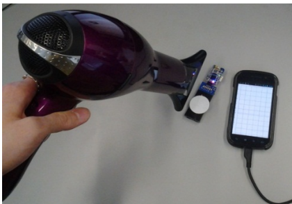
Figure 7. Testing temperature sensor data transmission
