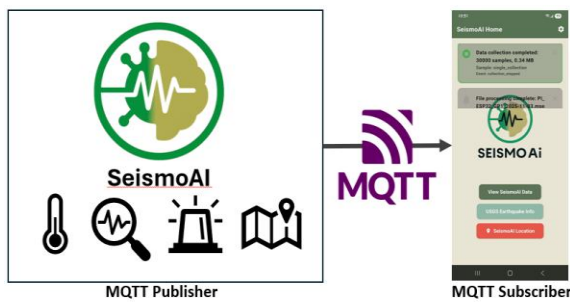
Figure 8. Mobile Application Architecture
