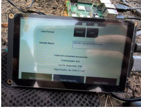
Figure 11. Touchscreen display showing recorded output. Note: Components were tested outside the final enclosure to confirm functionality before assembly
