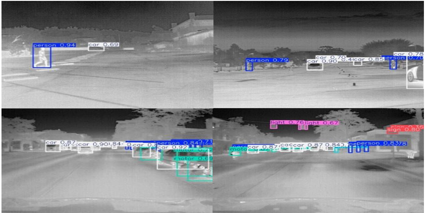
Fig. 2. Detection of on road objects along with their confidence scores. Different scenarios are tested: crosswalks, parking lots and intersections.
