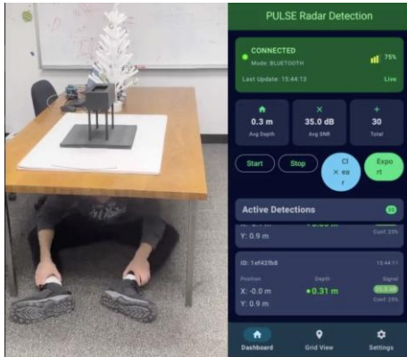
Figure 6. Testing with a human target through obstacles
